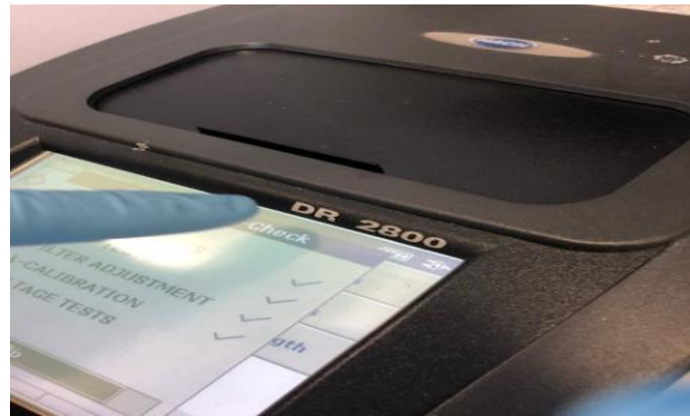
Figure 3: DR2800 Spectrophotometer for measuring COD.
