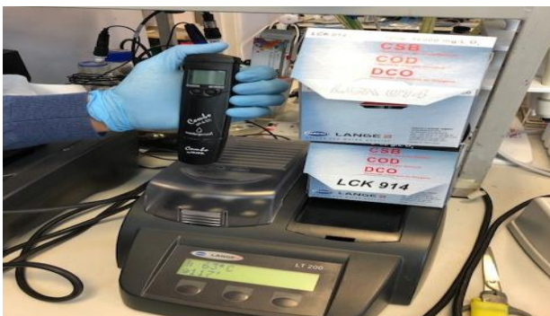
Figure 1: COD analysis, Digestion phase. LT 200 thermostat reactor.
