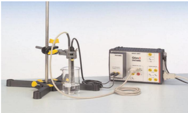
Figure 1: Cobra 3 device for measurement of pH and EC.
