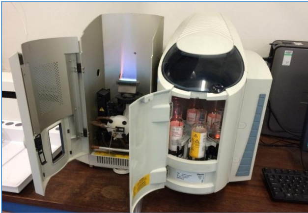
Figure 4b: Atomic adsorption spectrophotometer – sample under test.
